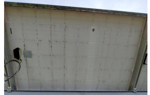
Example of PV module back sheet defect
