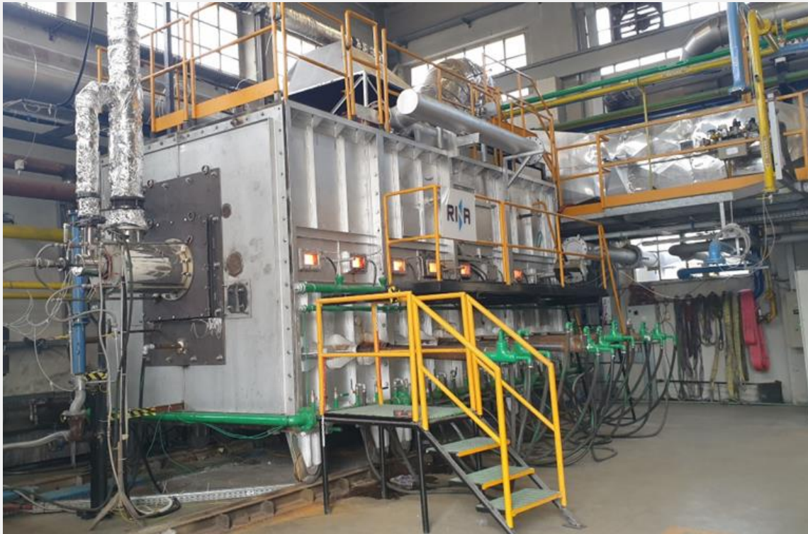
Furnace chamber: 2 x 2 x 6 m
